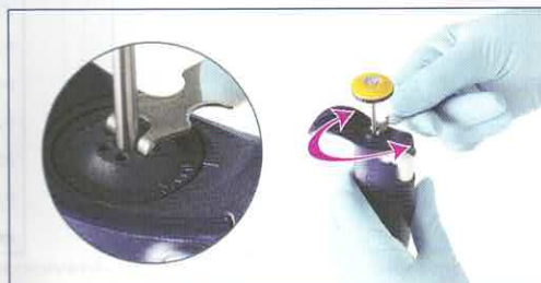
Figure 6 PIPETMAN ® L Fixed Model Adjustment Hold the key in the highest position to avoid banging it into the hook.
