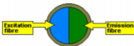
Figure 80 The end of the fibre optic accessory
