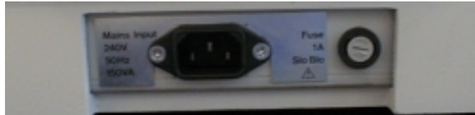
Figure 12 Mains connection and voltage plate
