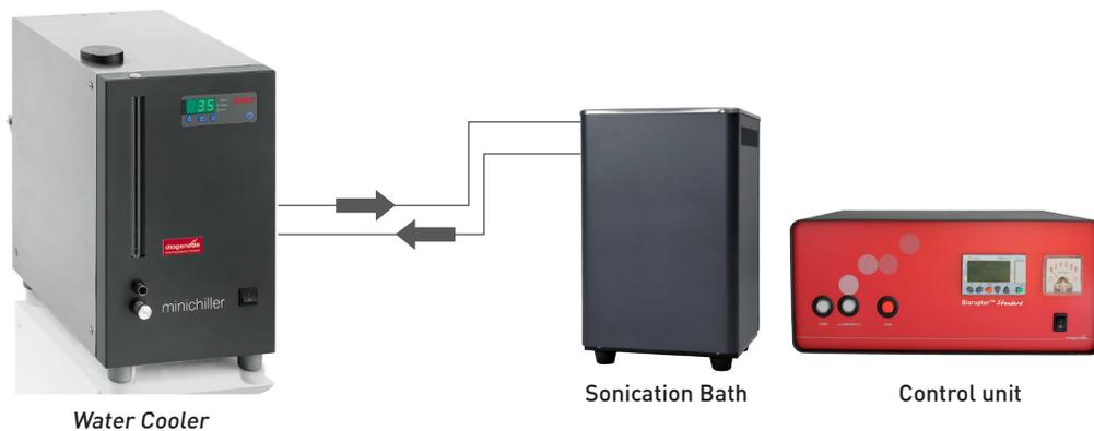
Fig 3. Setup of the Bioruptor® Standard in combination with the Water Cooler.
