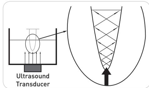
Fig 1. Propagation in 0.5 ml tubes and 1.5 ml tubes
