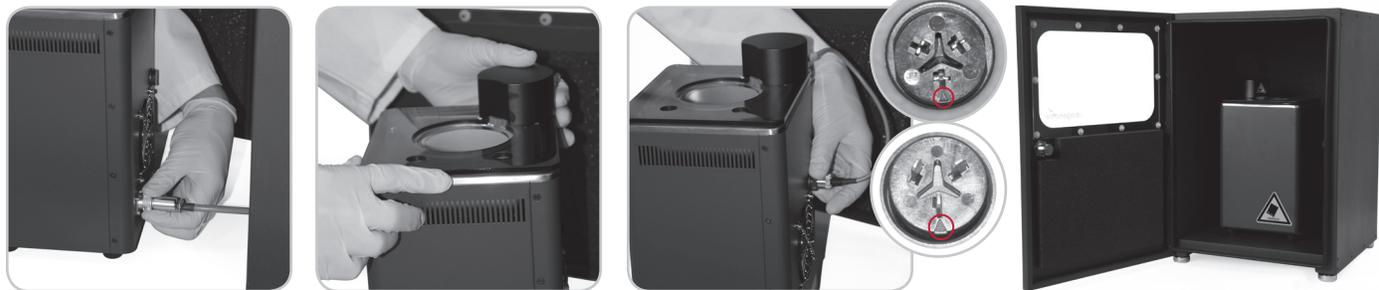
4. Plug the control unit cable into the sonication bath.
