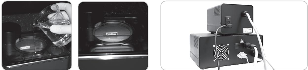
7. Fill the sonication bath up to the red fill line with distilled water only. Do not use deionized water!
