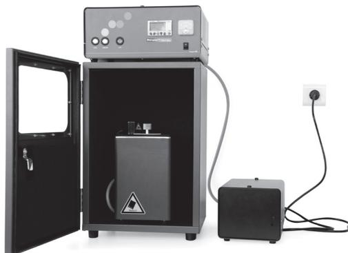
9. Place the control unit on top of the soundproof box. Plug the power cable into the outlet and switch on the power switch on the back of the control unit.
