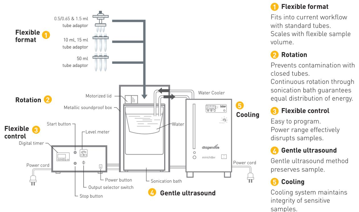
Fig 5. Schematic installation overview of the Bioruptor® Standard in combination with the Water Cooler.
