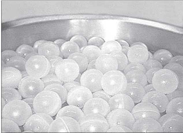
Picture 47: Floating balls in waterbath
