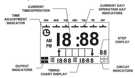
Figure 6 Optional Electronic Timer Display Detail
