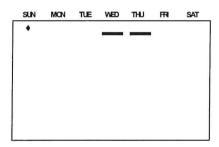
7. Press the **WRITE KEY** to enter this override into memory. The override will stay in the timer's memory for one week and a day (until the following Monday), after which the timer will operate in its previously set programming scheme.
