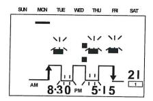
6. Using the h and m KEYS, set the span of time that the switch will be off 0:01 (1 minute). Press the WRITE KEY to enter this value into memory. Please note that the cycle-on or cycle-off time cannot be set to 0:00. The timer will display the complete operation for approximately one second, then the display will return to the initial PROG1 SET MODE DISPLAY. The number of available programmable operation steps remaining is displayed in the lower right hand corner.
