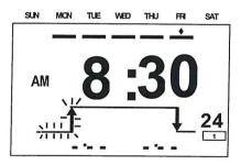
4. Press the WRITE KEY to enter this setting into memory. If the day, hour, and/or minute have not been set, the specified time and day will not be entered into memory when the WRITE KEY is pressed. Once the WRITE KEY is pressed, the timer will display the next available setting in PROG1. In this case, the timer will display the time the operation will stop.
