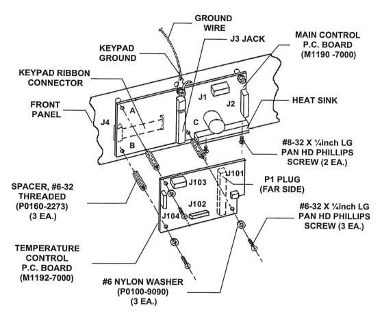
Figure 19 Temperature Board Replacement
