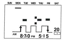
7. Set the MODE SWITCH to the RUN position to exit the PROG1 set mode.
