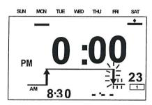
5. Using the h and m KEYS, set the time to 0:00 pm. Press the WRITE KEY to enter this setting into memory. The timer will display the complete operation for approximately one second, then the display will return to the initial PROG1 SET MODE DISPLAY, with the number of programmable operation steps remaining displayed in the lower right hand corner.
