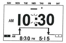
3. Open the lower drawer of the timer and press the CHECK KEY. Each time this key is pressed, the operation schedule is displayed in the sequence the operations are to be executed. The ON and OFF times for PROG1 are displayed, starting with the earliest ON time. Then the times set for PROG2 are displayed. After all the set times of both programs have been displayed, the timer returns to the RUN display.
