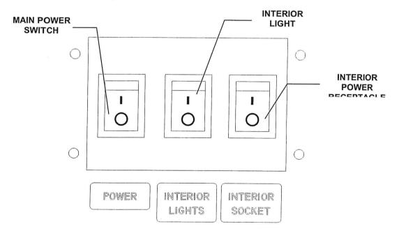
Figure 11 Switch Panel Detail
