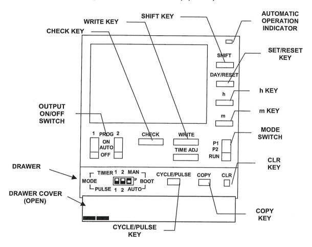
Figure 5 Electronic Timer (Optional) Detail
