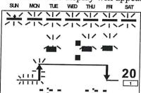
2. Press the **WRITE KEY**. If it is necessary to change the setting, do so with the appropriate keys and press the **WRITE KEY** to enter these values into memory. Each time the **WRITE KEY** is pressed, the programmed times are displayed in the order that they were set.
