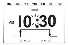
2. Hold down the **TIME ADJ KEY** for one second or more. An arrow and a flashing clock will appear under the word **SUN** in the display to signify that the timer is in **TIME ADJUST MODE**. The timer will stay in this mode for approximately one minute if no adjustments are made.
