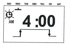
6. Verify that the settings entered are correct, and press the **WRITE KEY** to set the day and time. When the **WRITE KEY** is pressed, the arrow and flashing clock disappear from the display, and the timer is set to the displayed time at 0 seconds.
