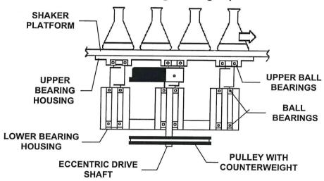
Figure 16 Bearing Housing Replacement
