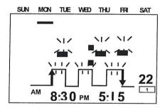
5. Using the h and m KEYS, set the span of time that the switch will be on to 0:02 (2 minutes). Please note that the cycle-on or cycle-off time cannot be set to 0:00. Press the WRITE KEY to enter this value into memory. The timer will then prompt for the cycle-off time.
