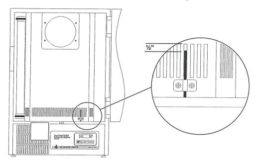
Figure 18 Temperature Sensor Adjustment
