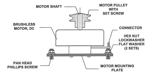
Figure 15 Motor Replacement
