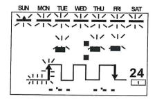
3. Using the SHIFT and SET KEYS, select the day of the week that the cycle operation is to start. In this example, the cycle is to be performed on Monday. Using the h and m KEYS, set the time the cycle operation will begin on Monday to 8:30 am. Press the WRITE KEY to enter this setting into memory.
