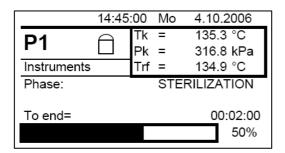
The sterilizer is in sterilization phase, 2 minutes before finish of this phase.
