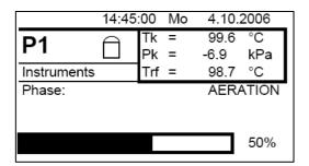
Pressure reduce is over, now the chamber is venting until reaching setpoint.
