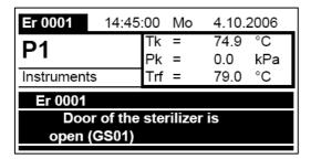
The program P1 was started but lid was not completely closed. So the device generates an error message. The error message can be cleared by pressing the Escape button if the cause of the error was cleared.
