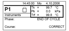
The program cycle has finished successfully. The sterilizer gives the result as correct cycle. Now the program needs to be quit by pressing the Stop button. Then the lid can be opened and the sterilization good can be removed from chamber.
