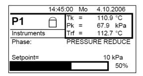
Sterilization phase has finished, now the chamber pressure will be reduced until reaching 10 kPa in chamber.
