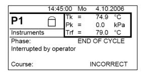
Before regular end of cycle a break was initialized maybe by hand or automatically. In case of automatic break an error message is additionally shown.
