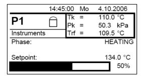
Deaeration has finished, the program is now in heating phase. Setpoint for finish of this phase is reaching the 134°C chamber temperature.
