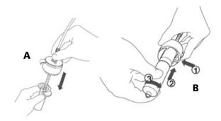
Figure 7: In 7a, Insert the plunger into the cap; and 7b Align and push cartridge into the cap, and then rotate the cartridge to secure it.
