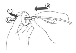
Figure 6: Press the lever and extend the plunger
