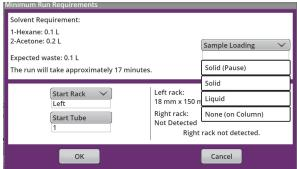
Figure 3: MINIMUM RUN REQUIREMENT screen and loading options
