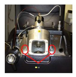
Figure 5-13 Ion source chamber
