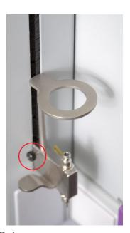
Figure 2-13 Location of the side hole to secure the SLCC ring support
