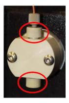
Figure 5-16 Check valve holder
