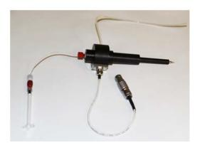
Figure 5-15 ESI probe with syringe
