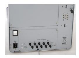
Figure 2-4 Location of external gas ports
