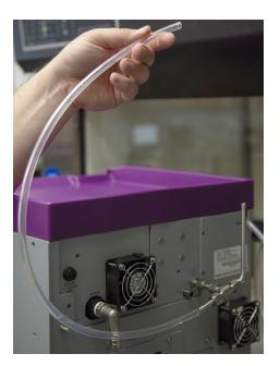
Figure 5-8 Line filled with 40 ml of acetone
