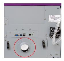
$Figure\ 2\text{-}10\ Location\ of\ the\ external\ exhaust\ port$
