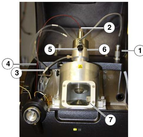
Figure 5-12 Removing the APCI probe
