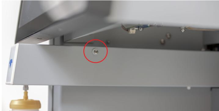
Figure 2-1 Remove screw holding the arm in place
