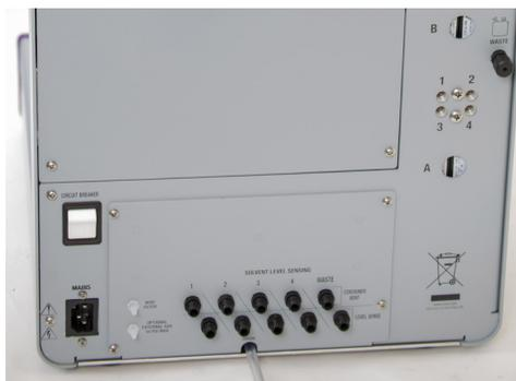
Figure 2-4 Location of external gas ports
