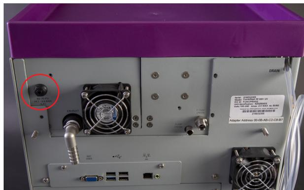
Figure 2-5 Location of ELSD gas port (Nitrogen input line circled)
