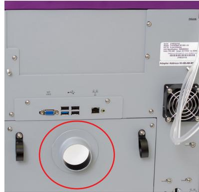
Figure 2-10 Location of the external exhaust port
