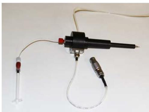
Figure 5-15 ESI probe with syringe
