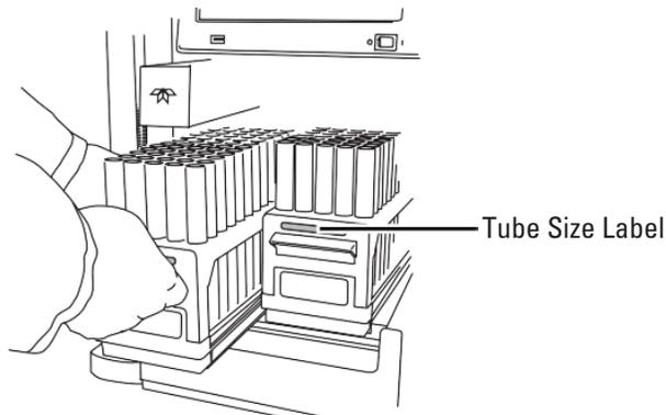
Figure 2-15 Inserting the collection tube rack
