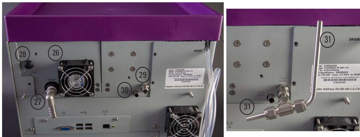
Figure 1-8 NextGen ELSD (back) and P-Trap Drain Vent Assembly
