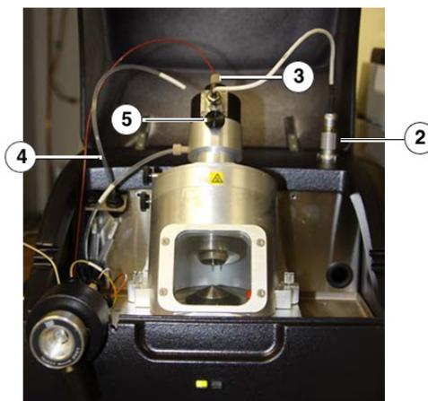
Figure 5-11 Removing the ESI probe
