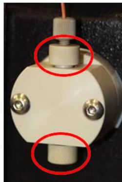
Figure 5-16 Check valve holder
