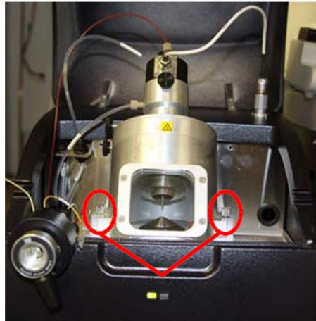
Figure 5-13 Ion source chamber
