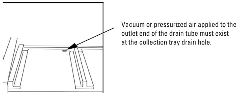
Figure 2-6 Fraction collection tray drain hole
