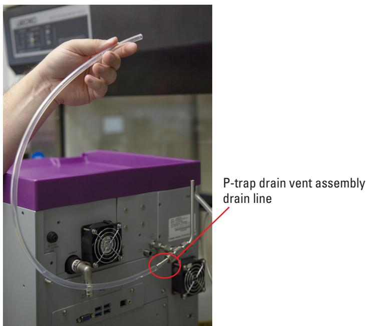
Figure 2-8 Keep liquid level lower than the top of the system
