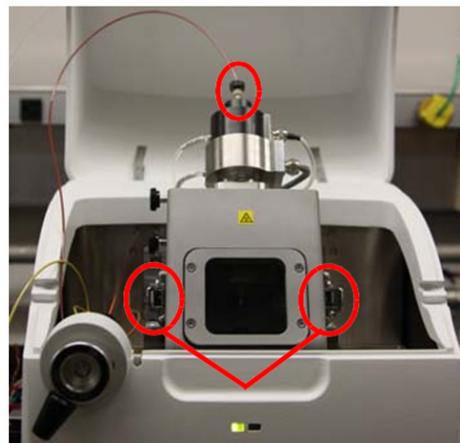
Figure 5-14 ESI and APCI removal from PurIon S and PurIon L
