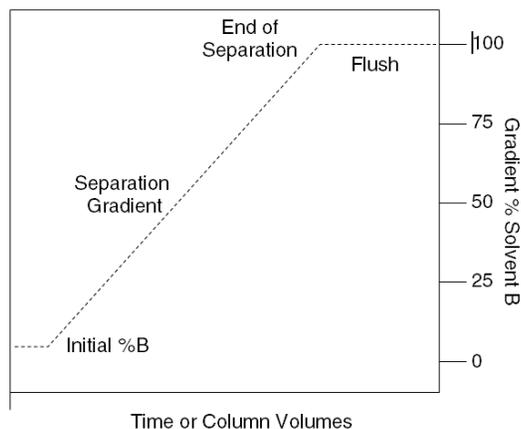
Figure 5-3 Default post-separation column and flow cell flush
