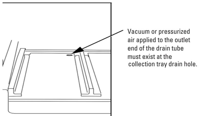
Figure 5-1 Fraction collection tray drain hole
