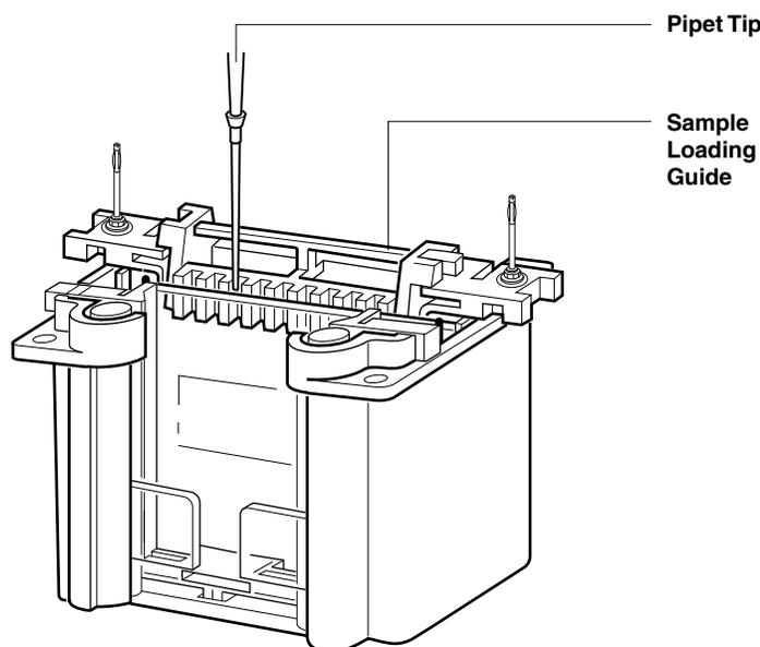
**Fig. 6. Using the Sample Loading Guide (patent #5,656,145).**
