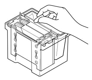
8. Put on the lid, plug the cables into the power supply, and run the blot. Refer to Section 3 for run times and voltage settings with various buffers.
