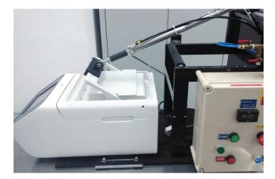
Figure 1. ProFlex PCR System instrument in "lid actuation robot". This testing involves repeated opening and closing of the heated cover to determine the lifespan of the lid mechanism.
