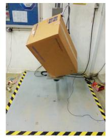
Figure 3. ProFlex PCR System shown in shipping box drop testing.
