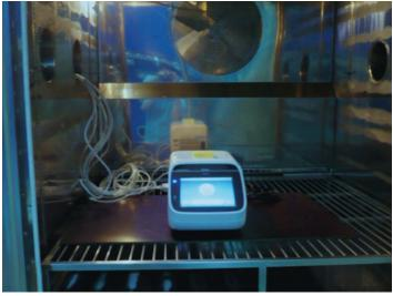
Figure 2. High-temperature testing of the Applied Biosystems<sup>™</sup> SimpliAmp<sup>™</sup> Thermal Cycler inside an environmental chamber.
