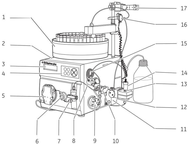
Figure 1.1: The main parts of the instrument.
