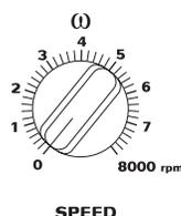
The variable-setting knob is used to set the drive speed, in 200-rpm increments, up to 8000 rpm. For precise speed adjustments, the ACCU-SET button can be pressed as the speed knob is turned until the required speed appears on the RPM display. The centrifuge will accelerate to the set speed and maintain that speed for the duration of the run.<sup>1</sup> ACCU-SET can be adjusted at any time during a run.
