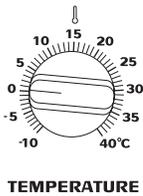
This knob is used to set the operating temperature between –10 and +40°C in 1°C increments. (Recommended operating temperature range is from –5 to +25°C.) A thermistor in the chamber regulates the compressor to maintain chamber temperature  $\pm 2^\circ\text{C}$  of the set temperature.<sup>2</sup>
