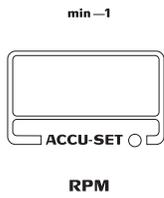
When centrifuge power is turned on, the display shows “0000.” During the run the display indicates actual rotor speed to the nearest 10-rpm increment. If the run is shut down prematurely due to one of four conditions (see Section 4, TROUBLESHOOTING), the diagnostic message “8880” will be displayed.
