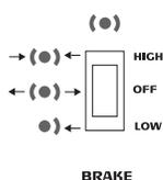
This switch is used to select the brake mode used during deceleration. Refer to the appropriate rotor manual for acceleration and deceleration times for available rotors under various conditions. The three positions of the switch provide:
