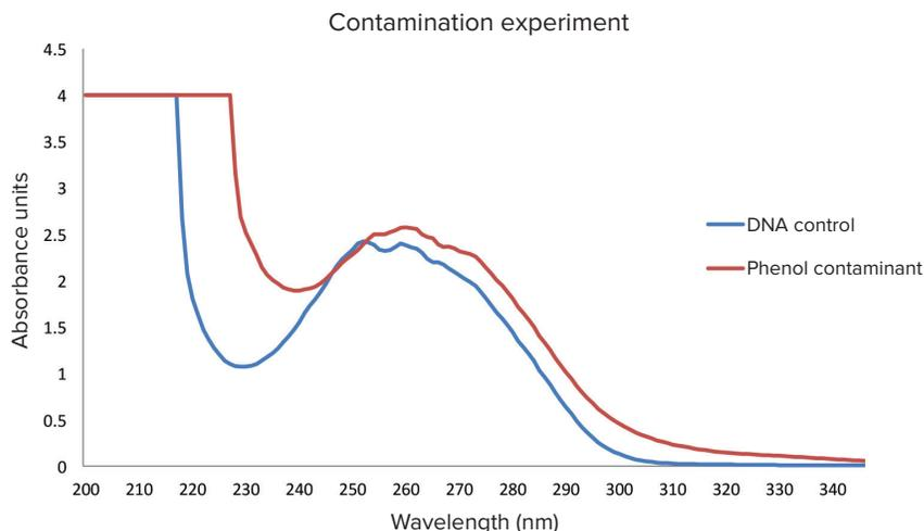
**Figure 5. Contaminant experiment.** Phenol-contaminated samples and an uncontaminated control were assayed using the Wavescan function. Wavescan traces were graphed and overlaid using Microsoft Excel. There is a definitive increase in absorbance at the 230 nm mark.
