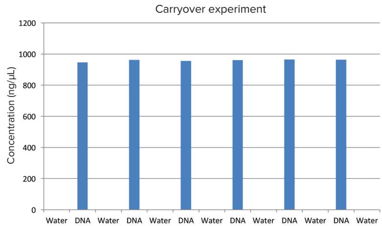
**Figure 1. Sample carryover.** Alternating measurements of calf thymus DNA and water were performed on the micro-volume port. Data were graphed on Excel. The data comprising this graph are shown in Table 1.
