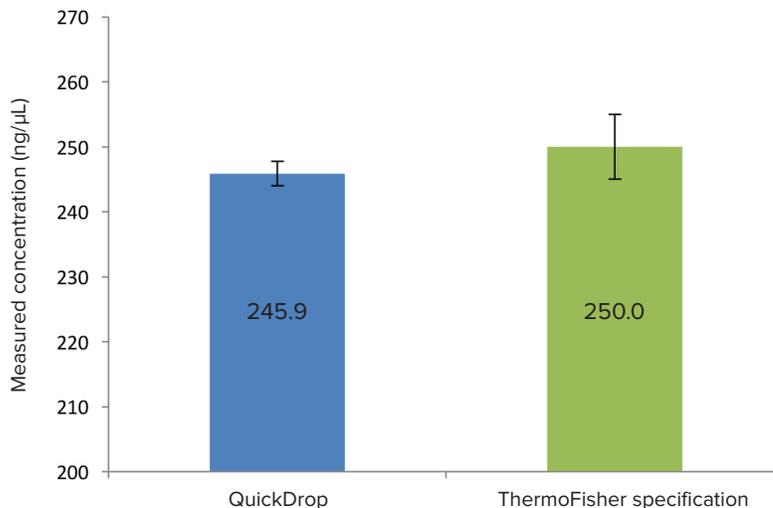
**Figure 4. RNA validation experiment.** 250 ng/ $\mu$ L RNA Control was measured on the QuickDrop to compare results to ThermoFisher's NanoDrop validation results ( $n = 4$ ). The measured RNA concentration ( $245.9 \pm 1.9$  ng/ $\mu$ L) falls within ThermoFisher's specified range ( $250.0 \pm 5.0$  ng/ $\mu$ L).
