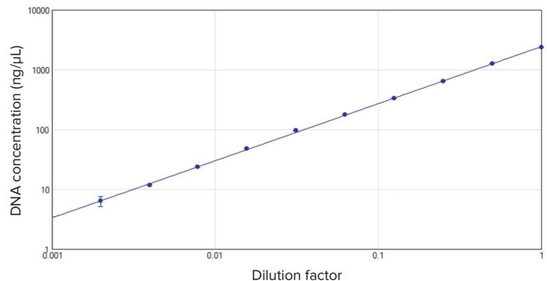
**Figure 2. Calculated DNA concentration vs. dilution factor.** A 2-fold dilution series of calf thymus DNA starting from 2500 ng/µL shows the relationship between the dilution factor and the DNA concentration reported by the QuickDrop. The curve demonstrated excellent linearity with a  $r^2$  value of 1.000.
