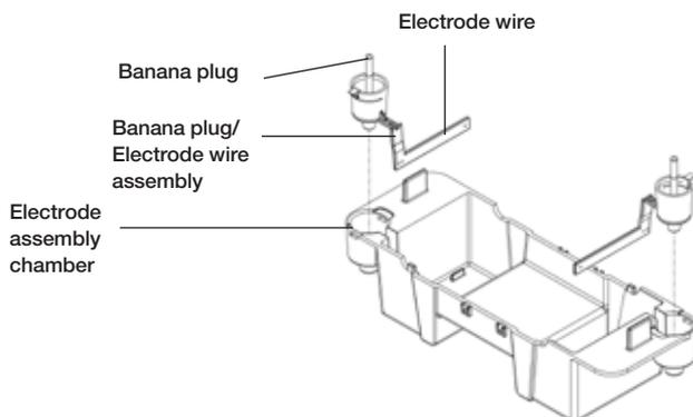
Fig. 4.1. Removal of banana plug/electrode wire assembly.
