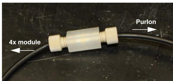
Figure 4-3 Coupler for connecting 4x tubing
