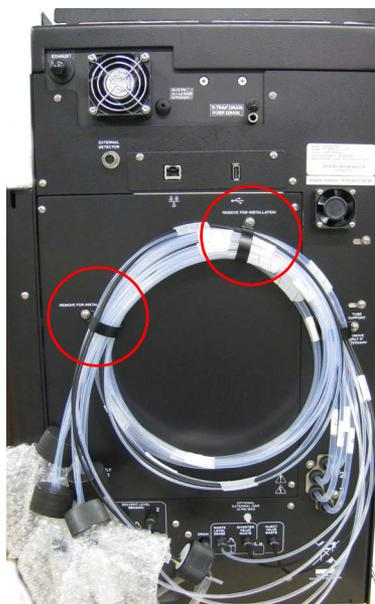
Figure 2-4 Remove the two shipping clamps indicated above
